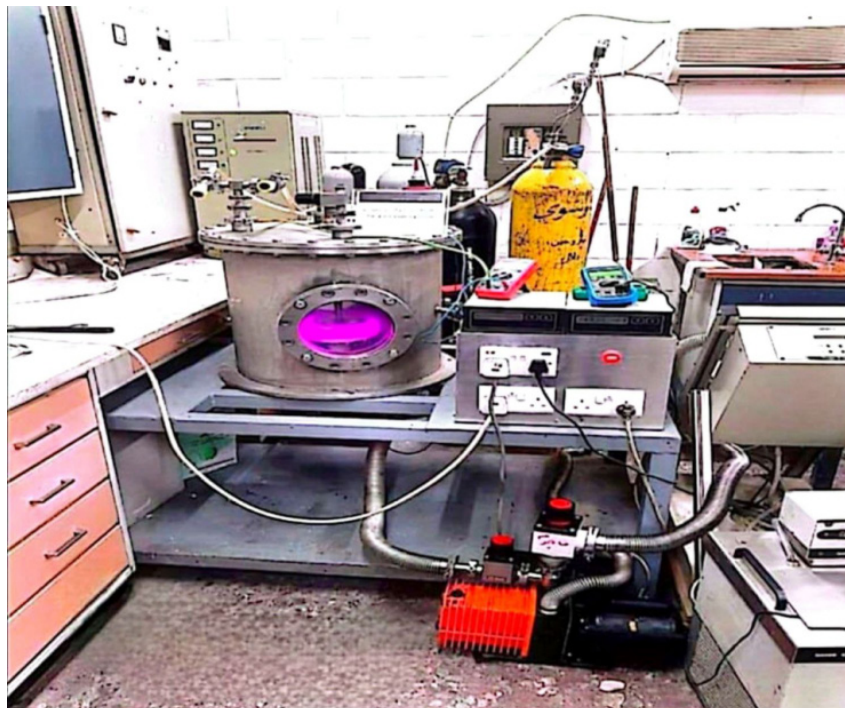
Fig.1 plasma Sputtering system
