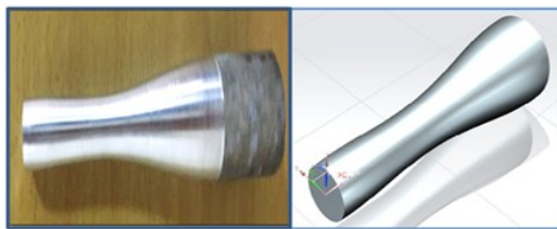
Figure 4. Workpieces CAD vs. CAM
