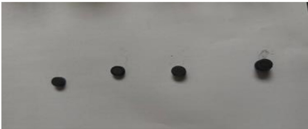
Fig. 2. Compressors made of nickel base and carbon nanotubes (CNTs) reinforcement.
