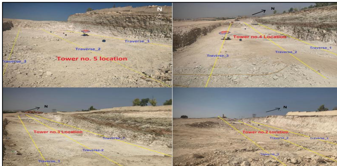
Figure 3. Twelve survey profiles (traverses) were conducted across four residential towers.
