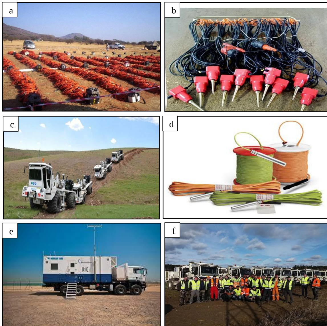
Figure 4. Seismic field equipment at the Hariri field, Erbil, Iraq, including (a- line cables, b- geophones, c- explosives cables, d- vibrators, e- dog room, f- seismic crew).
