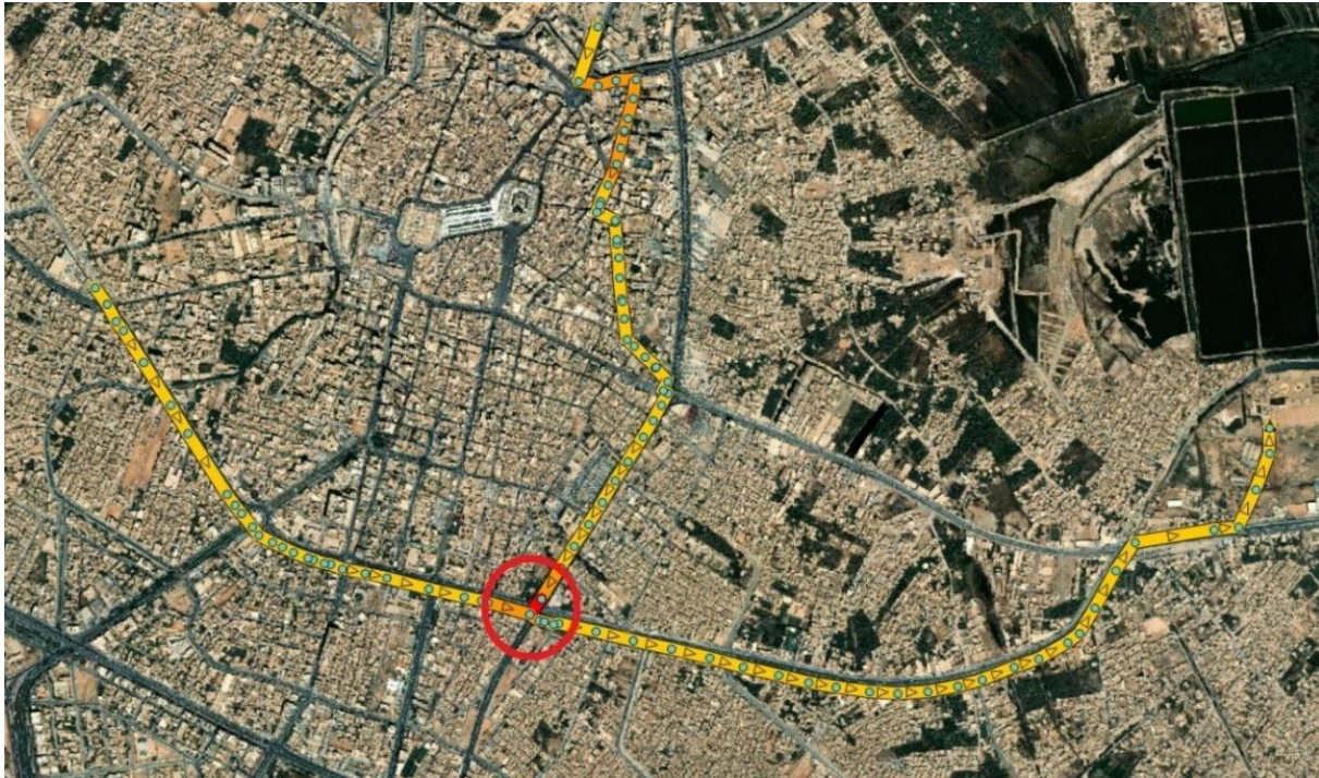
Figure 16. C26 pipe reaching 100 % capacity during 20 mm/h rain event.
