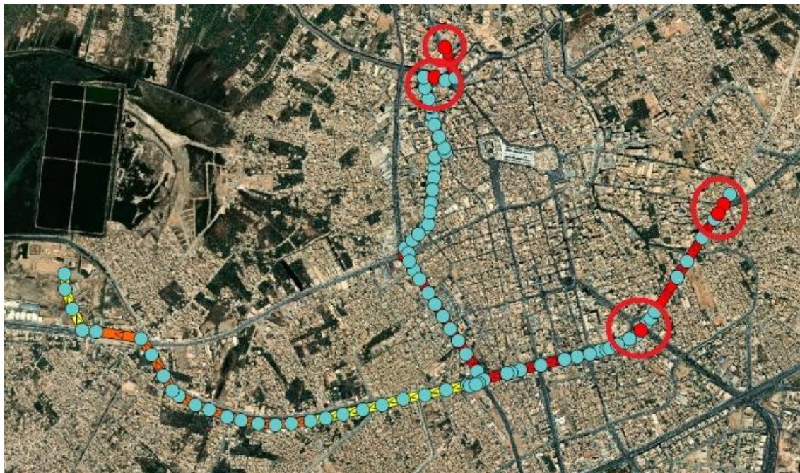
Figure 23. Flooding places (40 mm/h rainfall event).
