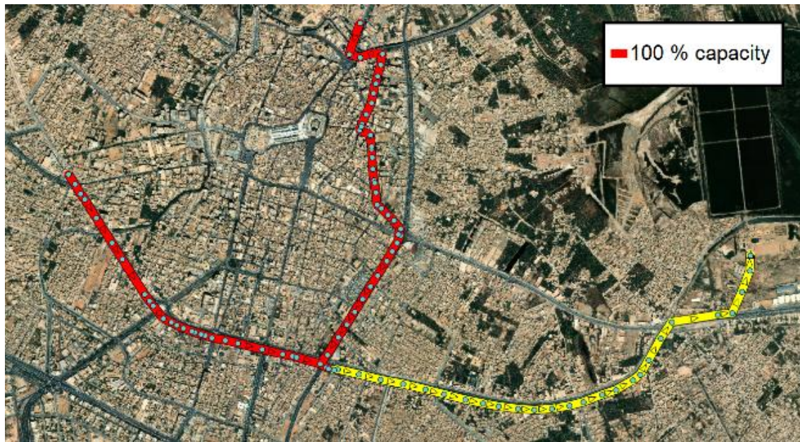
Figure 20. Pipe capacity situation under 25 mm/h rainfall event.
