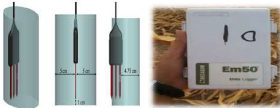
Figure 1. Mechanism for placing sensors in the soil.
