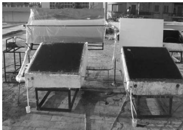
Fig. 3. Modified and standard solar stills.
