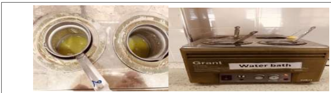
Figure 3.Heating a Sample of Available Boron in Water Bath at constant Temperature
