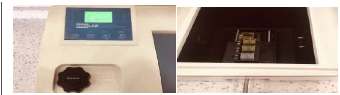
Figure 7. place the sample in the spectrophotometer to measure boron at a wavelength of 540 nm, using the transmission mode.
