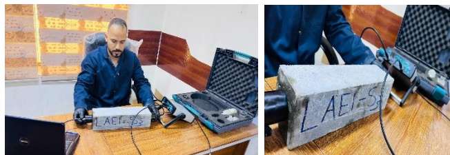
Figure 16. UPV test for A-EPSC samples.
