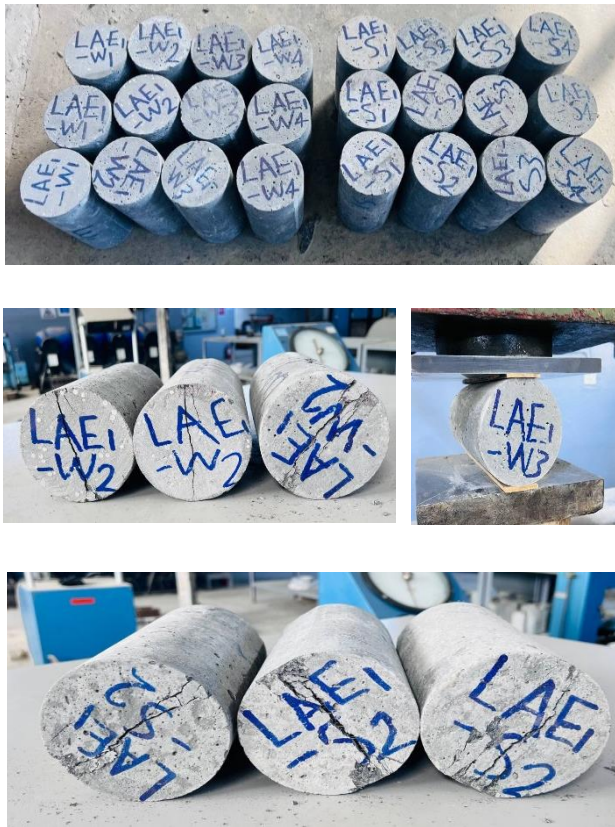
Figure 12. Samples subjected to the splitting test.
