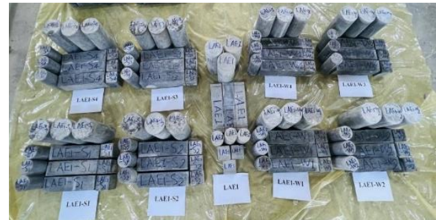
Figure 5. Prepared LWC samples for the tests.
