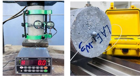
Figure 13. Modulus of elasticity tests (static and dynamic).
