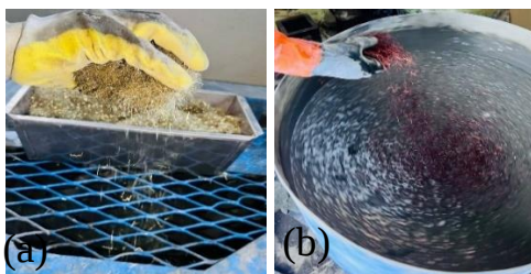
Figure 3. The method for incorporating (a) micro-steel fiber, (b) waste copper fibers.
