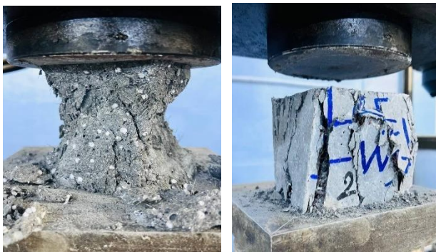
Figure 9. Compressive testing of the Cubes sample.
