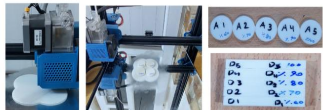
Figure 7. The 3D printer was fabricating Prose Functionally Gradient Materials (PFGM).
