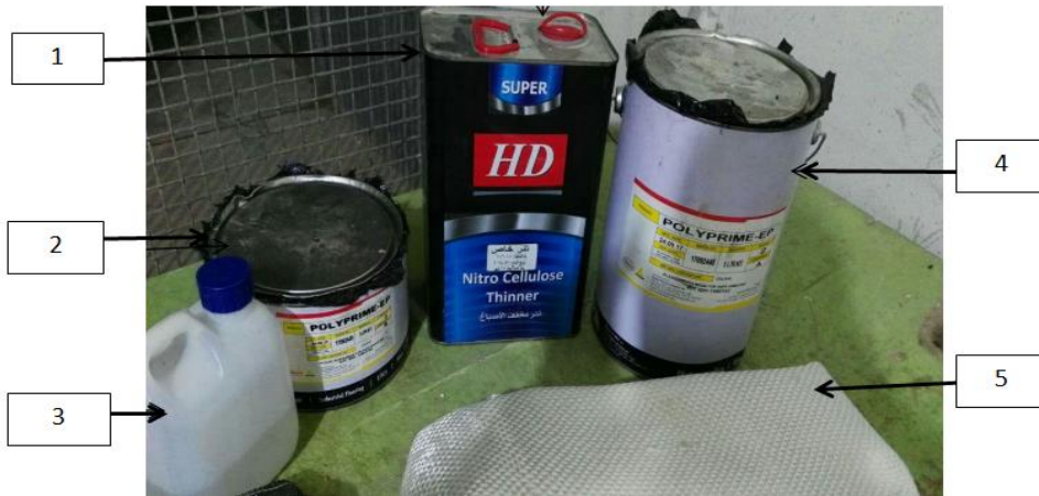
Figure (6): Materials used for preparing a tensile specimens: (1) Cleaning material, (2) Hardner, (3) Isolation material, (4) Epoxy, and (5) Woven glass fiber.
