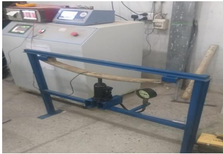
Figure (12): Experimental test for calculation the induced stresses and deflections.
