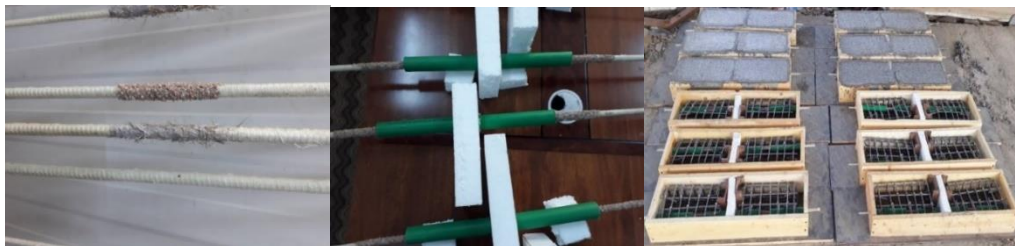
Fig. 2. Specimen preparation and casting process
