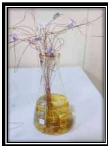
Fig (2) Chemical etching process of the CR-39 detector.
