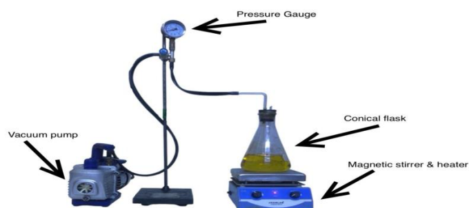
Figure 5: Oil Blending Process.
