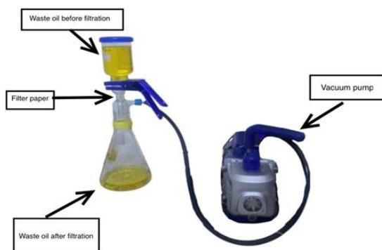
Figure 1. Filter System of WSO/WCO.
