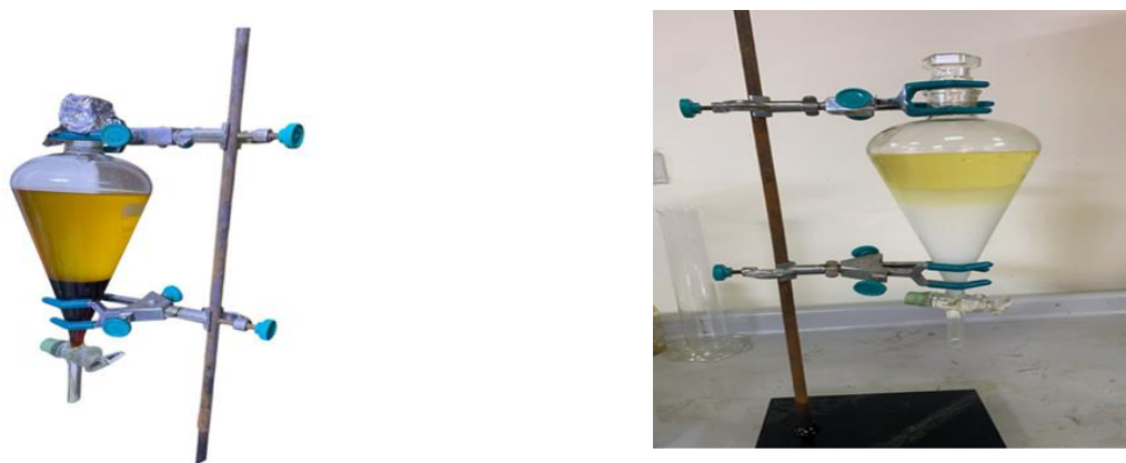
Figure 4. (a) Fatty esters and glycerin in the separation funnel, (b) Fatty esters and water in the separation funnel.
