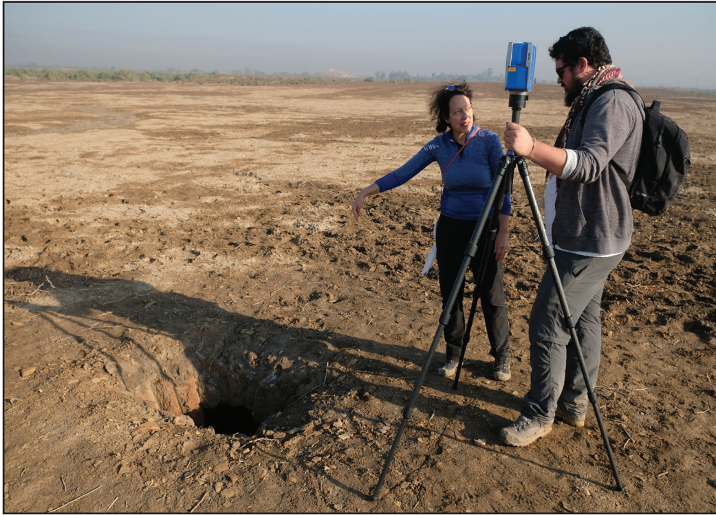
Fig. 5, Terrestrial Laser Scanning for documenting the vaulted tomb
