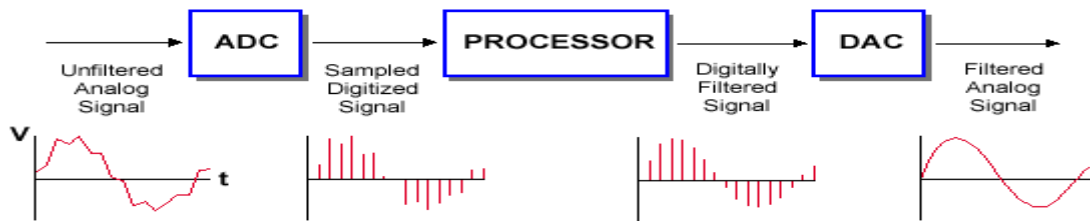
Figure (1): A block diagram of a basic digital filter[2]
