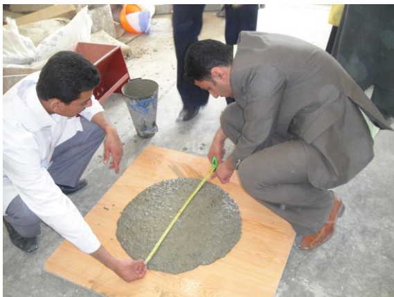
Fig.( 3) Slump flow of SCC– 0 minute after mixing
