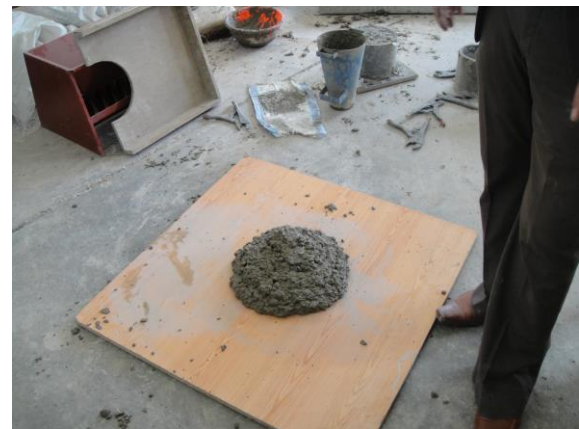
Fig.( 4) Slump flow of SCC– 30 minutes after mixing
