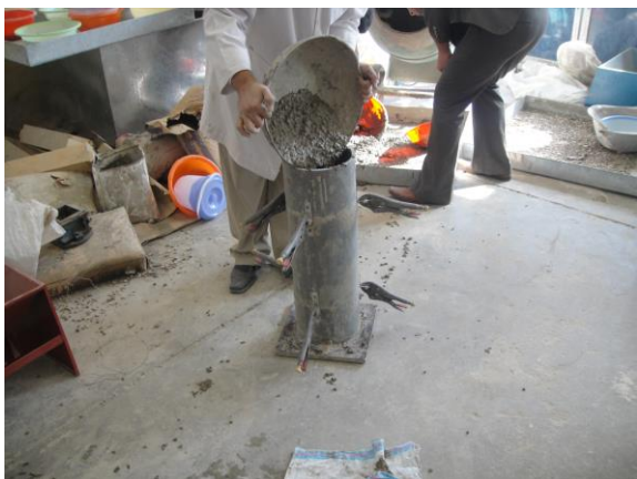
Fig.(7) Column segregation resistance test of SCC
