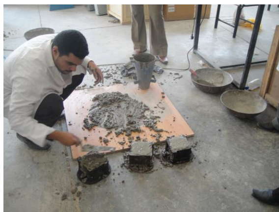
Fig.(8) SCC lost its ability to flow into all spaces within the mold
