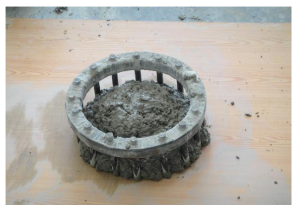
Fig.( 4) Slump flow of SCC– 30 minutes after mixing
