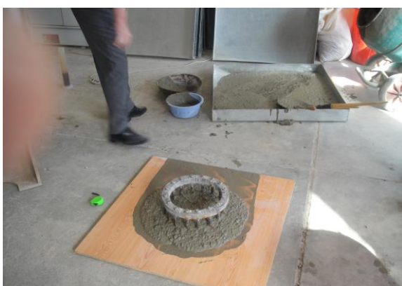
Fig.( 3) Slump flow of SCC– 0 minute after mixing
