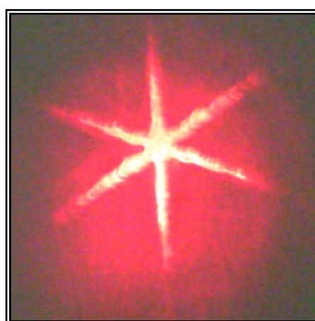
Fig . 18 : Diffraction pattern of triangle aperture as shown by a digital camera HD.
