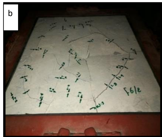
Plate 6: Crack pattern of 3Dtextile fibres 6mm, a) One layer. b) Two layers.
