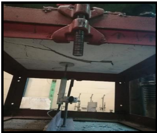
Plate 4: Bottom failure of SCMs fibre reinforced plate.
