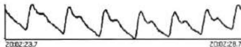
Fig.(3): Pulsatile signal obtained when IR or red light is transmitted through the finger.
