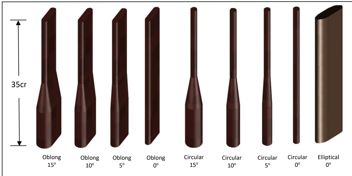
Fig. 3. Sketch of the oblong, circular and elliptical piers model.
