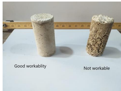
Fig.5 The effect of mix workability on specimen's quality
