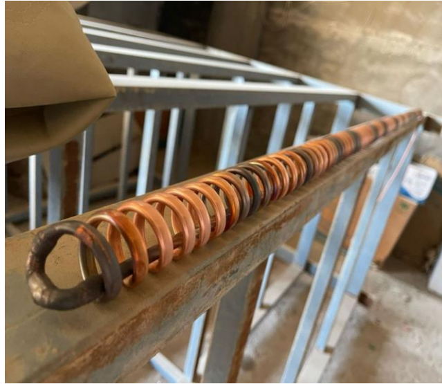
Fig. 7. Copper tube spiral coil
