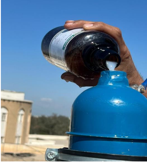
Fig. 9. Filling tubes with nanofluid
