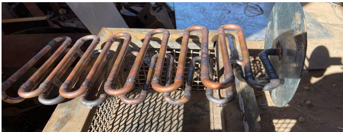
Fig. 8. Copper tube installed inside the tank
