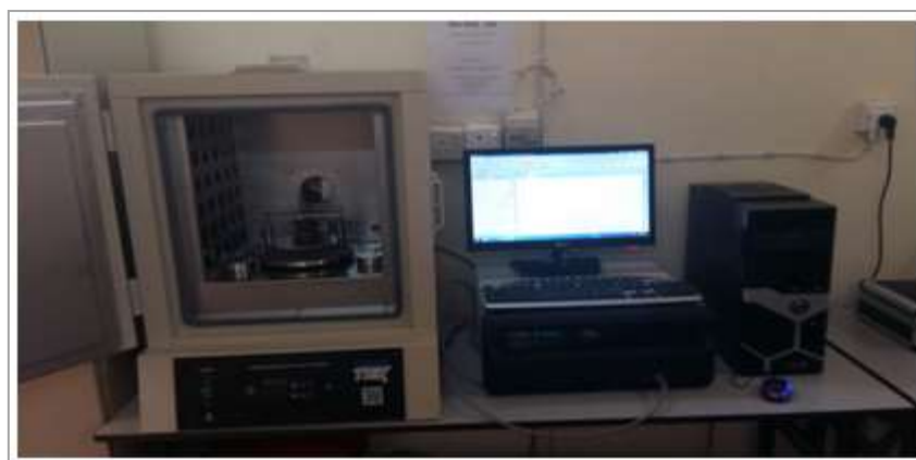
Figure (4) Hot Disk apparatus with samples
