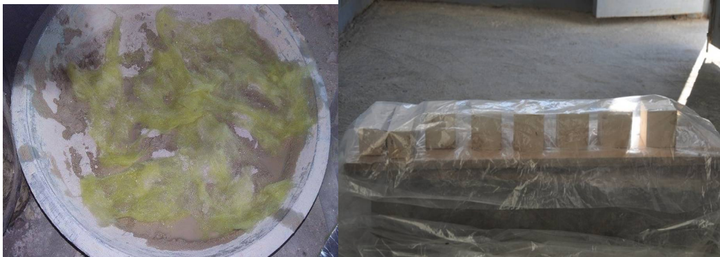
Figure 2. The processes of adding glass wool to the gypsum mixture and curing of the gypsum samples
