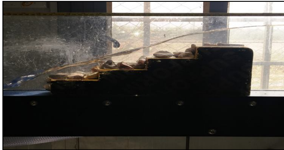
Fig.(11): Application of rough steps for the Models No. 7, No.8, and No.9.
