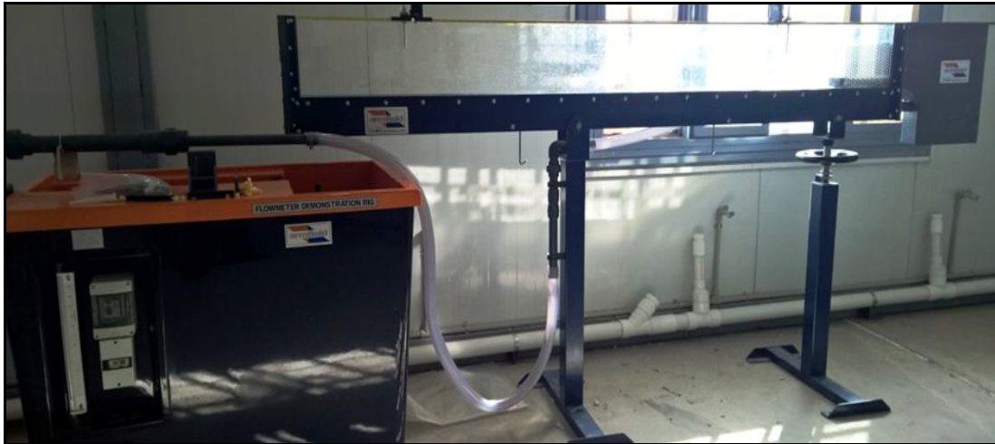
Fig.(1): The ARMFIELD flume used for the experiment.
