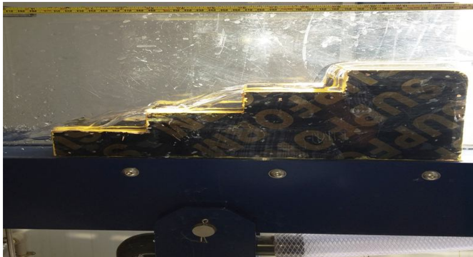
Fig.(4): Nappe flow.
