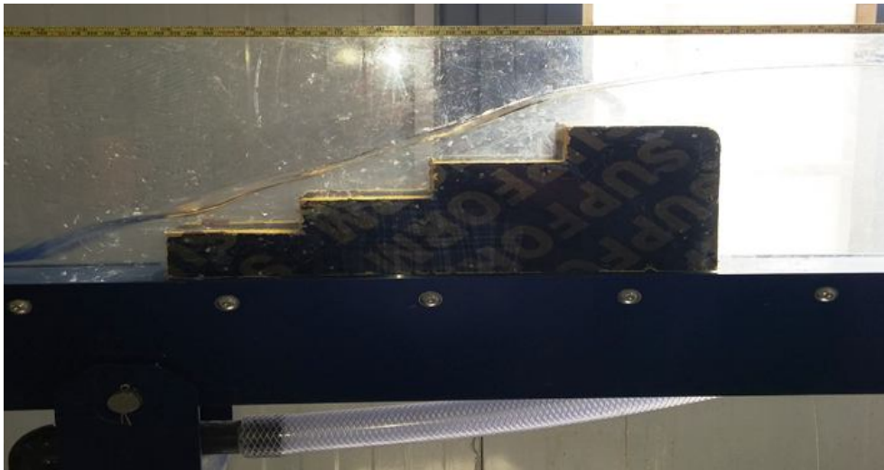
Fig.(6): Skimming flow.
