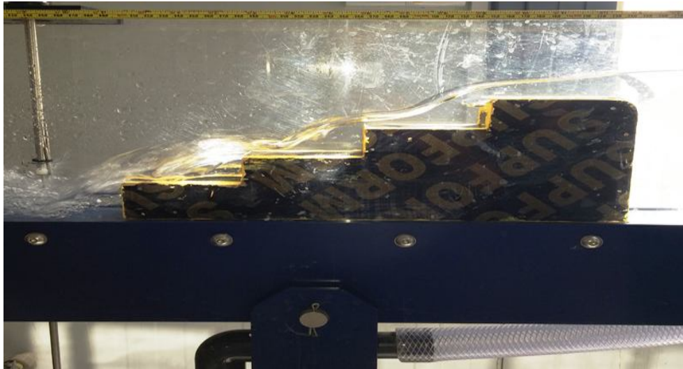
Fig.(5): Transition flow.
