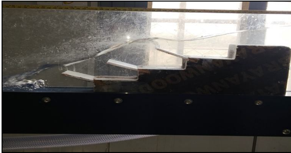
Fig. 13: Application of the inclined end sill steps for the Models No. 10, No.11, and No.12.
