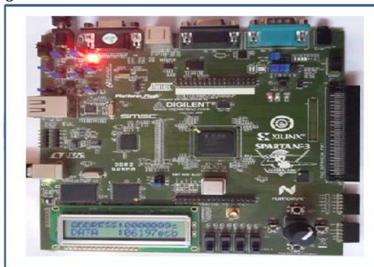
Fig.15. Fibonacci sequence program Results on Xilinx Spartan-3AN starter kit which in last value shows on LCD
