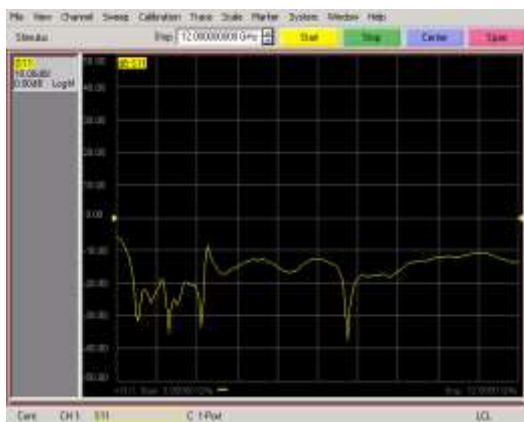
Figure 10: Shows a photograph of measured S11 of the practical connection of the Taconic TLY-5 antenna
