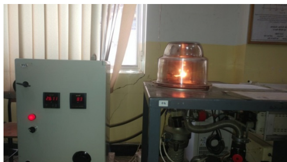
Figure 5: Thermal evaporation unit using in the study
