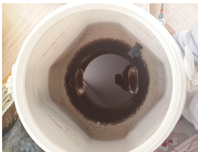
Figure 3: Precipitation of copper salts on the surface of container when pH=8.
