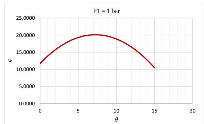
Fig. 9 the relationship between equivalence ratio and angle \theta .
