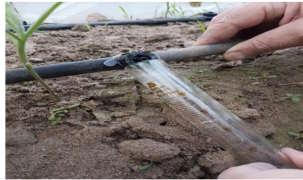
Fig. 3. cylinder to measure the emitter discharge.
