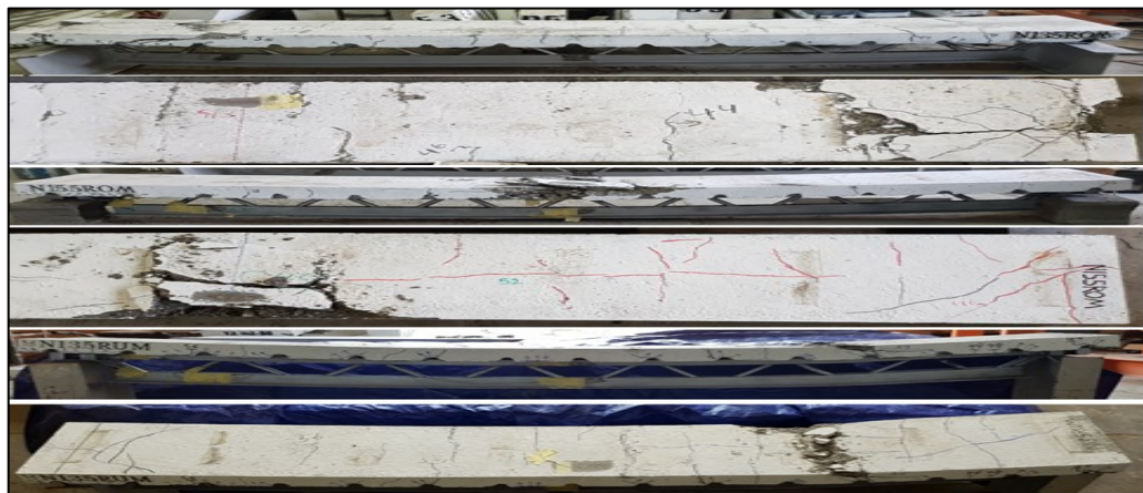
Figure 9: Composite joist specimens at failure.
