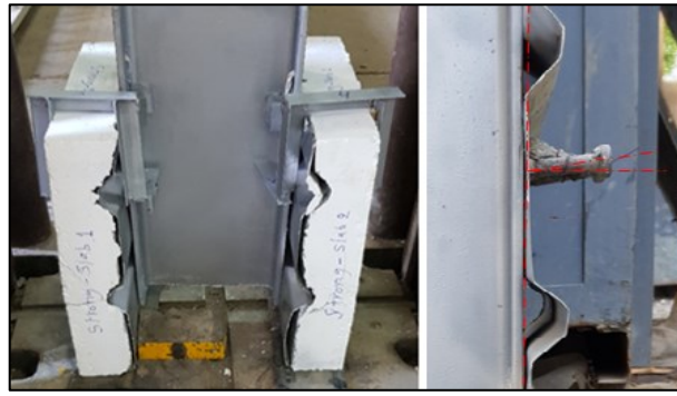
Figure 11: Typical cracking pattern and stud deformation of push-out test specimen
