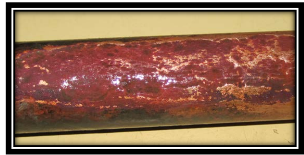
Fig.2. Pitting corrosion of tube wall,
