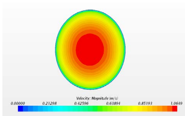
Fig. 17. Outlet Face Velocity magnitude in turbulent flow
