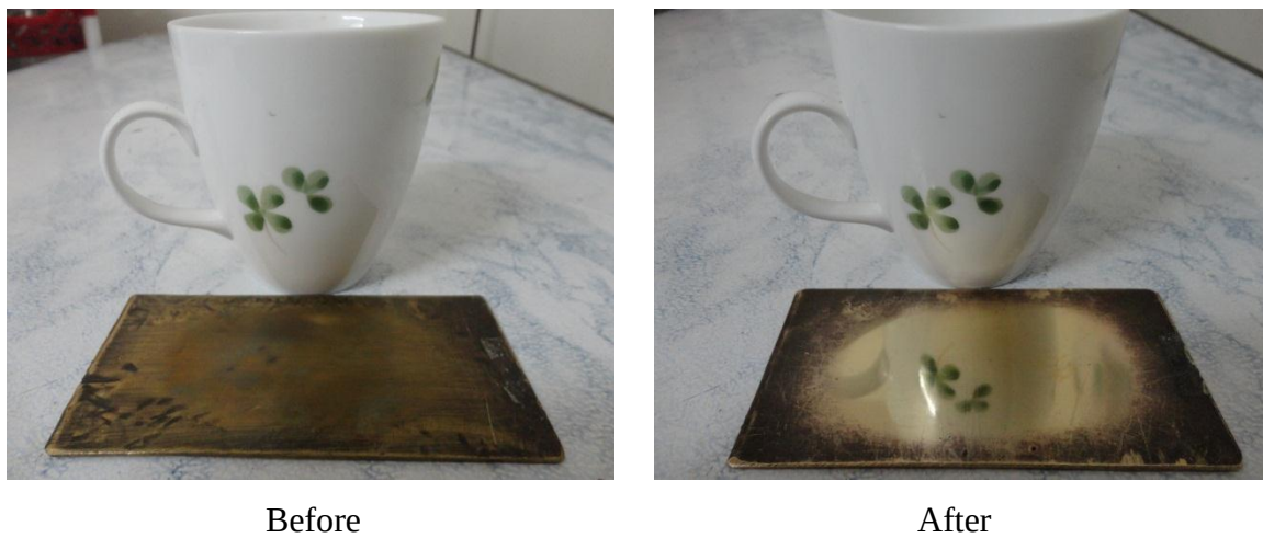
Fig (19): Photographs of workpiece finishing, speed= 525rpm; coil current= 1.5Amp; volume= 4cm 3 ; gap= 2mm.
