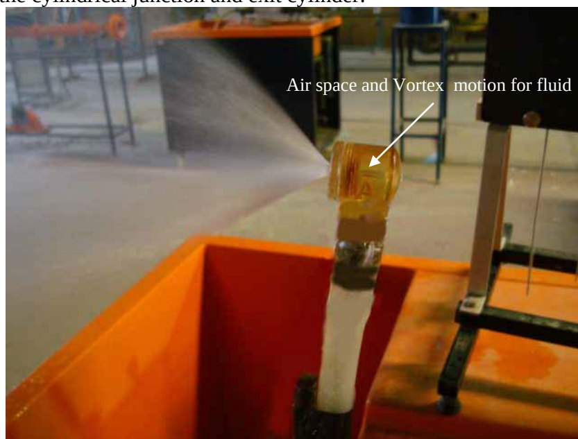
Fig.(1) Air Washer of the present work shows the vortex in the center of cylinder with no fluid.
