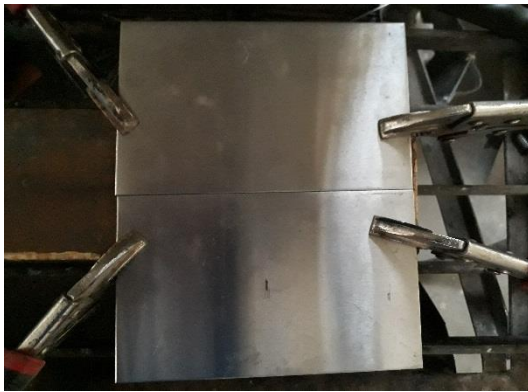
(a) Before welding
