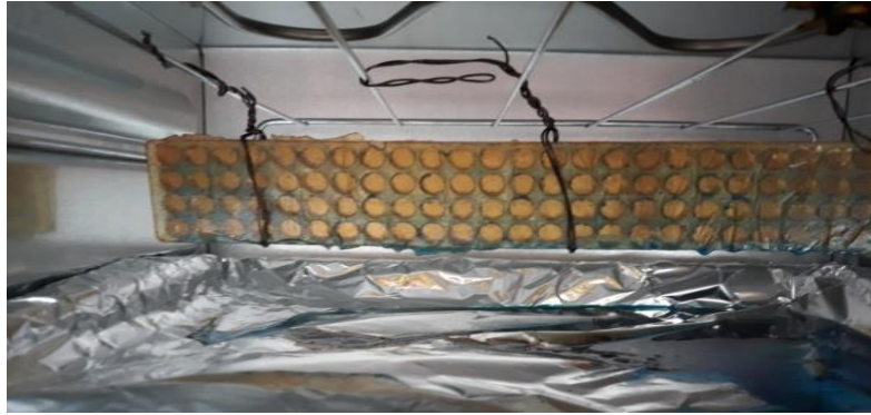
Fig 4: wax eliminated by gravity under (90-110 °C) temperature condition.
