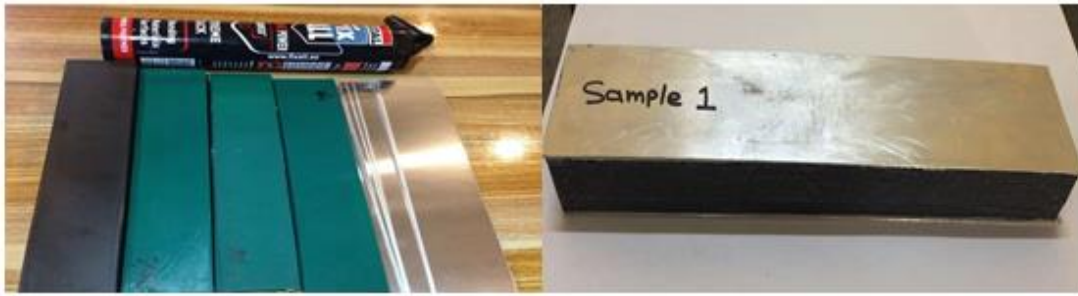
Figure 5: FG sandwich specimens with porous metal core
