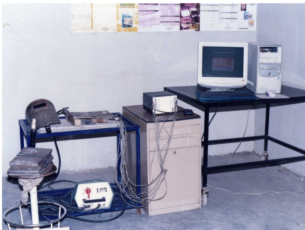
Fig. 8 . Data Acquisition System Frame and View for plates welding
