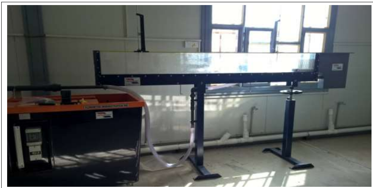
Fig.(1): The ARMFIELD flume at Al- Qadissiya University / College of Engineering.
