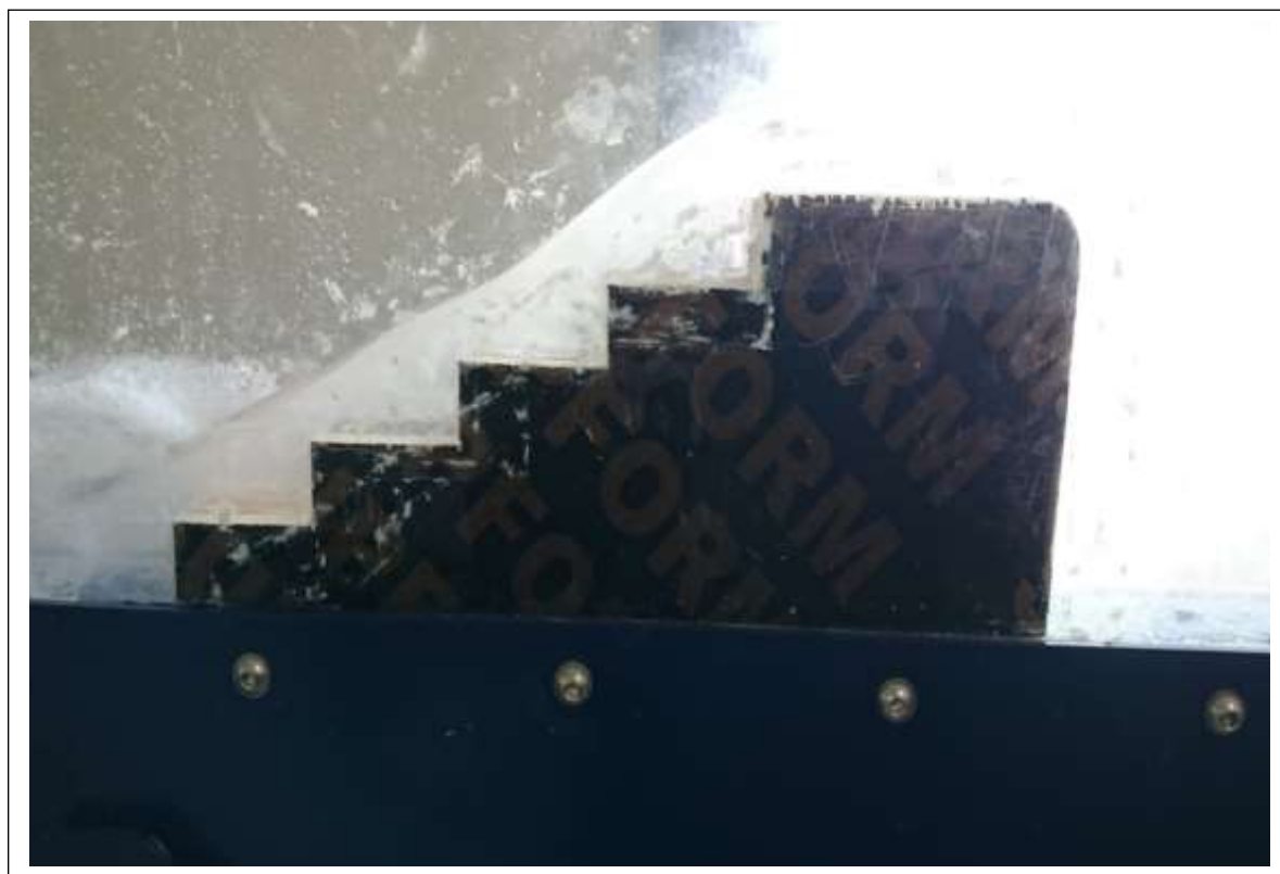
Fig.(5): Skimming flow.
