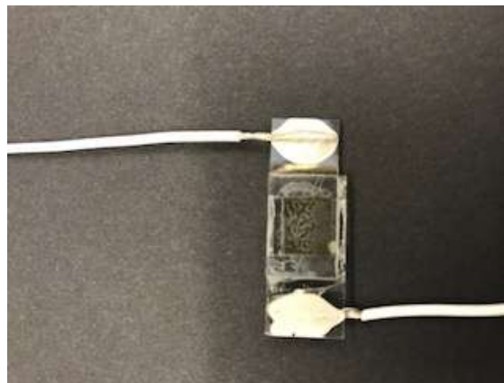
Fig. 6: The cell of PDLC (5CB doped with chitosan) doped with SBB dye.
