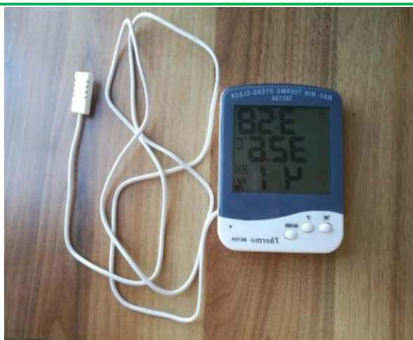
Picture (1): Sensor used to measure the relative humidity of the environment
