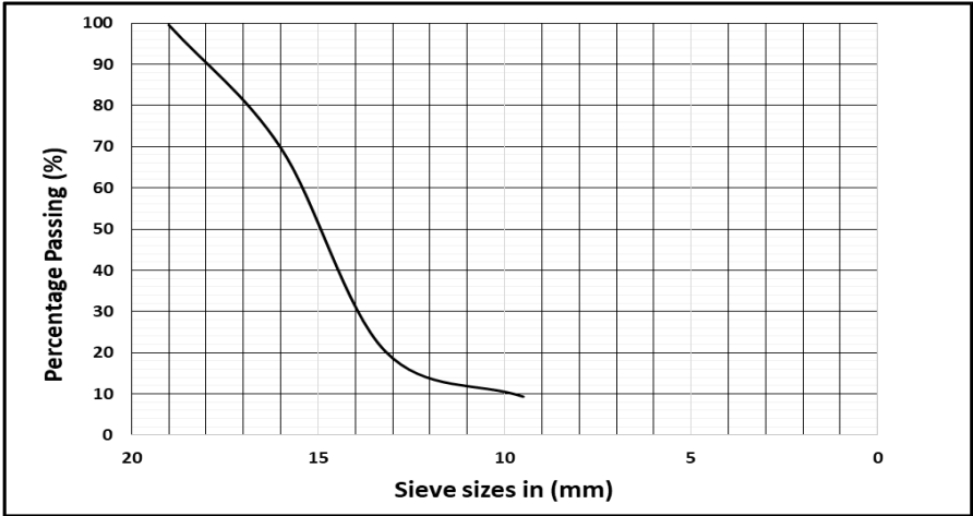
Figure 3: Grading curve of UPKS
