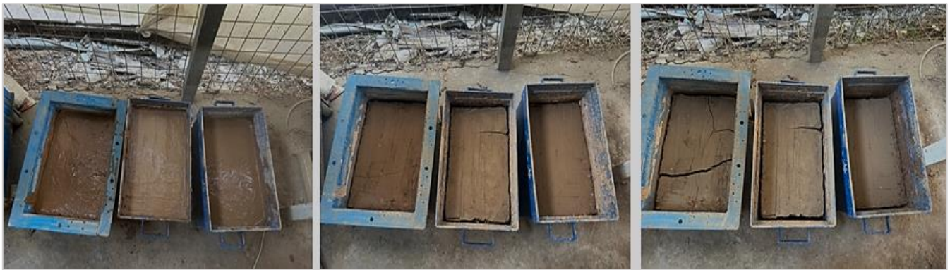
Figure 8: Photographs of the crack network developed in response to desiccation
