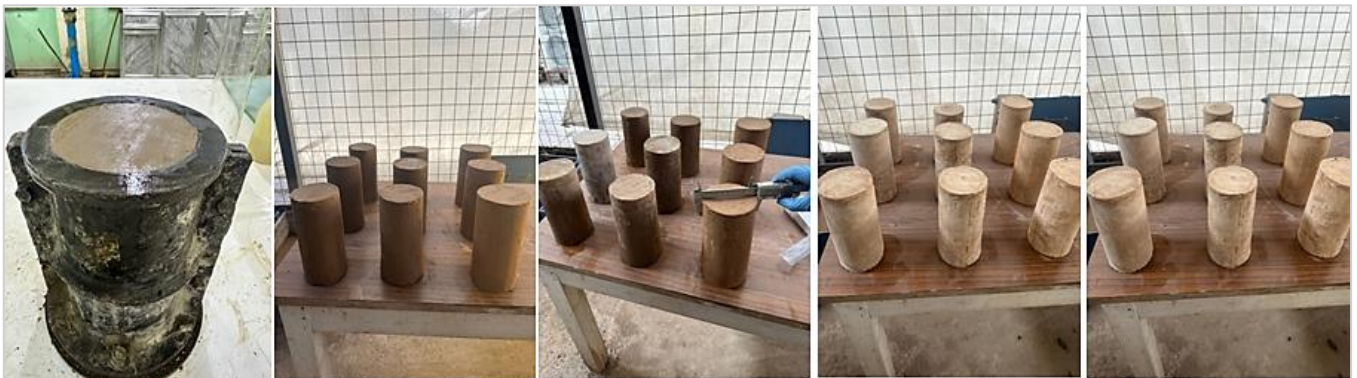
Figure 9: Photographs of the drying stages to calculate volumetric shrinkage
