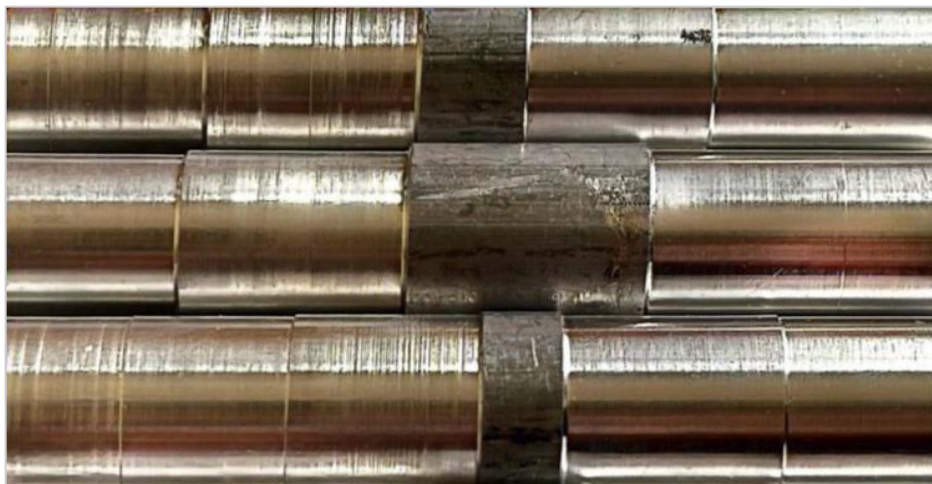
Figure 6: Finished sample after the turning machine process
