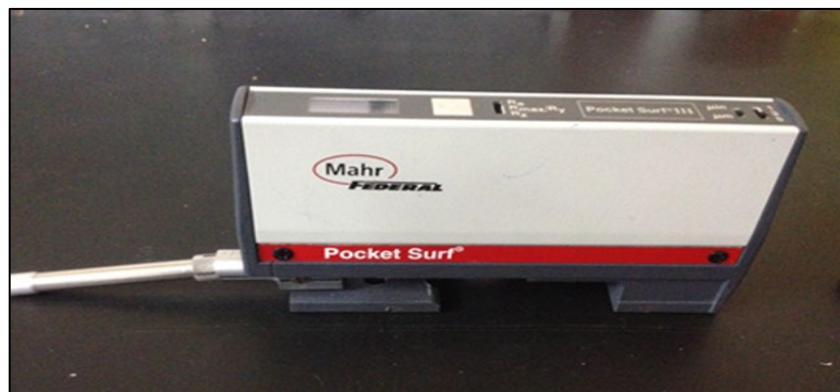
Figure 4: Profile-meter for measuring (SR)
