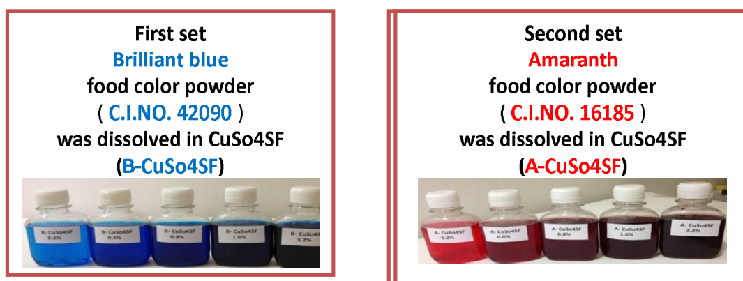
Figure (1): Sets B(CuSo 4 SF) and A(CuSo 4 SF), the following concentrations was prepared for each solution (0.2%0.4%0.8%1.6%,3.2%) wt./vol.
