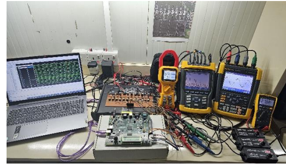
Figure 7. Experimental Setup of the seven-level multilevel inverter
